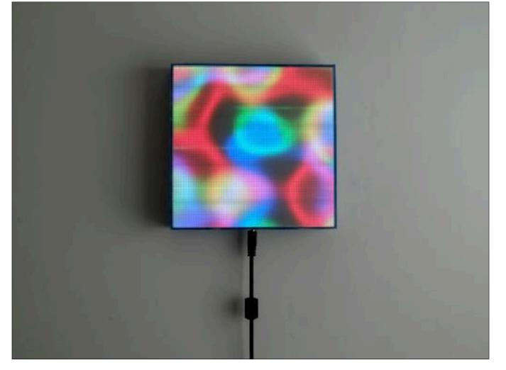
Works really well — **guaranteed no flickering** Simple **Linux library** that takes 64x64 32BPP RGB and does **massive bit-shifting**, writing to /dev/fb0 to send data out line by line. App simply sees a **flat RGB** frame-buffer Plasma, fractal animations
