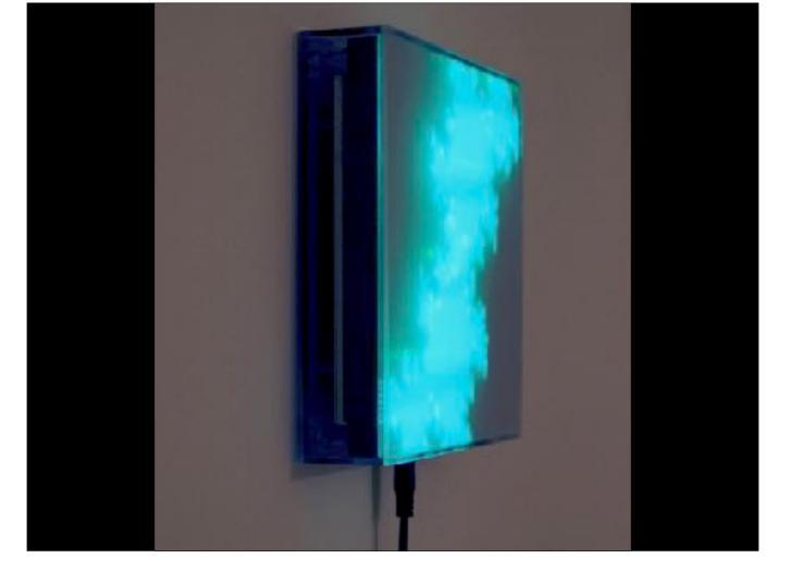
The **realtime Julia set fractal** was pretty smooth on the STM32, but super smooth on 1GHz CPU I haven't hacked **DOOM** to use it yet :) 177Hz, 11BPC/33BPP — **entirely flicker free** no matter how heavily loaded network/CPU is! **0% CPU overhead**
