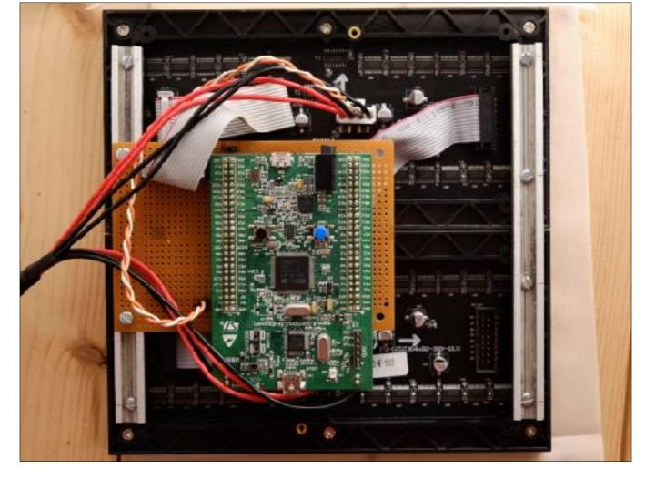
First proper go — driven from **STM32** Big shift register Clock data in for a whole row, then latch — example later Full-colour RGB — you have to do the PWM/brightness control by hand
