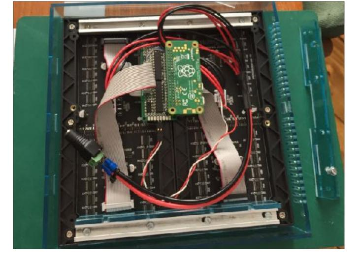
Little bit of protoboard — 74'245 to drive 5V Extremely cheap! Interface costs less than 1 beer Can see the acrylic case I started to build for it... **Glueing acrylic and trying to get it NEAT, OMG painful**
